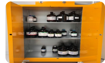
Installation of hazardous materials storage cabinets in the laboratory
