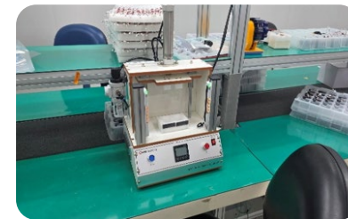
Installation of safety covers for small press equipment
